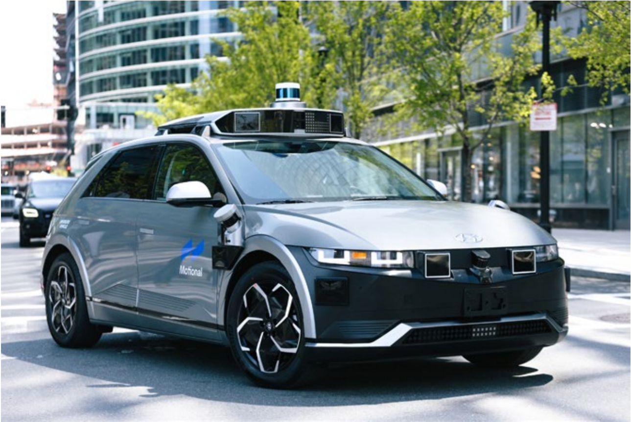
Motional's IONIQ 5 robotaxi, an autonomous vehicle equipped with sensors and onboard AI computing to keep passengers, pedestrians, and surrounding vehicles safe. Image credit: Motional.
