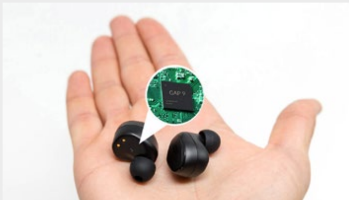
GAP9 processor, an advanced AI processor combining embedded AI and signal processing in wireless earbuds. Image credit: GreenWaves.
